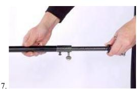
Slide the adjustable leg inside the panel leg with the divots facing the thumbscrew. When choosing the height of leg, be sure the thumbscrew seats in one of the divots. Divots are 1" apart for easy indexing.
