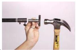
Take provided adapter and make sure the screws are "clear" inside (you should be able to slide your finger inside and not feel anything). Slide the adapter on the panel leg. IMPORTANT! The thumbscrew/set screw should be facing towards the inside of the opposite panel leg with the setscrew towards the panel and thumbscrew towards the foot. Place the T-Shape Installation Tool inside the adapter.
