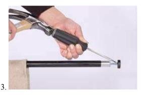
Remove the leg insert (white piece inside panel leg) by screwing in the leveler and using the screwdriver and hammer on the leveler to tap it out (insert and leveler will come out together). IMPORTANT! Replace strap, if there was a strap on this leg (next to seam of cover)
