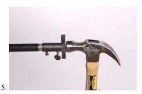
Tap the T-shape tool with the hammer until the adapter just touches black vinyl. Rotate and turn the T-shape tool to remove. (If stuck tap out with the hammer) REPLACE the T-shape tool inside the adapter. (The T-shape tool helps clear the dimples on the inside of the leg with initial entry, Second placement ensures leg stays round when adapter is tightened).
