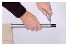
Slip supplied cutting guide over panel leg, under carpet, until it hits crossbar (horizontal bar at the bottom of the panel). While holding the cutting guide tightly, use razor knife to cut the black vinyl around the base of the cutting guide, and then again to the bottom end of the leg. Peel off piece of black vinyl and REMOVE cutting guide.
