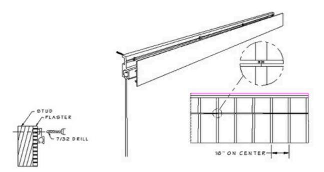
We provide 7 x 2" x #8 phillips-head deck screws with each 80" section of track. The Track is designed so that the ends will coincide exactly with the wall studs as illustrated above however, we do realize that this is not always the case.
